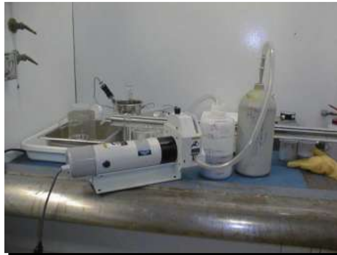
Peristaltic Pump Set Up
